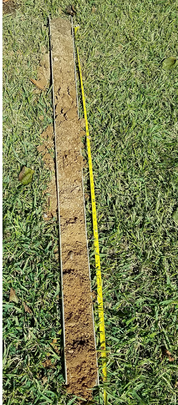
Figure 4. Bojac (or possibly State) soil profile bored and evaluated by Daniels & Whitehead on October 6, 2022, at the HR AREC demonstration garden area. This soil was observed at two locations (see Appendix C), one located next to the local weather station and raised beds area and at a second location pictured here just east of Diamond Springs Road. The soil is well drained with > 40'' to seasonal saturation and supports a wide-array of upland plantings in this immediate area and the nearby arboretum. Note: Lighter colored areas in this image were due to the soil drying down in the sun during the description period and were all \geq chroma 3 when excavated moist. The C horizon encountered here at > 40'' was a gravelly sand.
