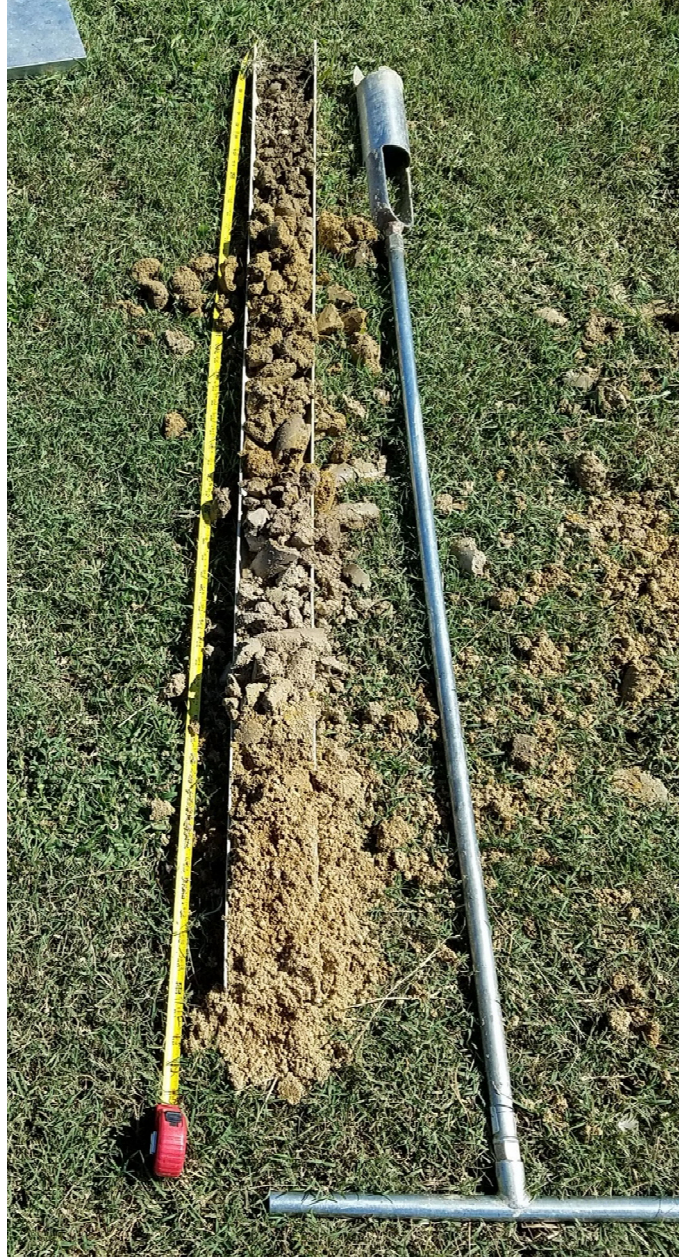
Figure 3. Tetotum soil profile bored and evaluated by Daniels & Whitehead on October 6, 2022, at the HR AREC research plot area. The majority of active research plots at the AREC are located on this moderately well drained soil type moderately well drained conditions with a depth to the seasonally saturated zone of 18 to 30". The auger shown is 60" for comparison.
