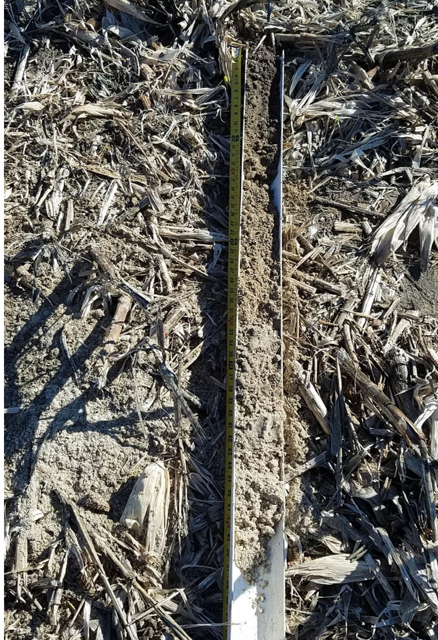
Figure 2. Munden soil profile bored and evaluated by Daniels & Whitehead on October 6, 2022, in the NE corner of the Brenneman tract. Note the “browner” hues in the subsoil down to ~30” indicative of moderately well drained conditions. This profile was much sandier in the subsoil than others we collectively observed over multiple field days.
